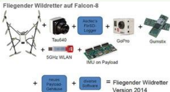
Image: How it works: technical components. Source: Wildretter F-C
